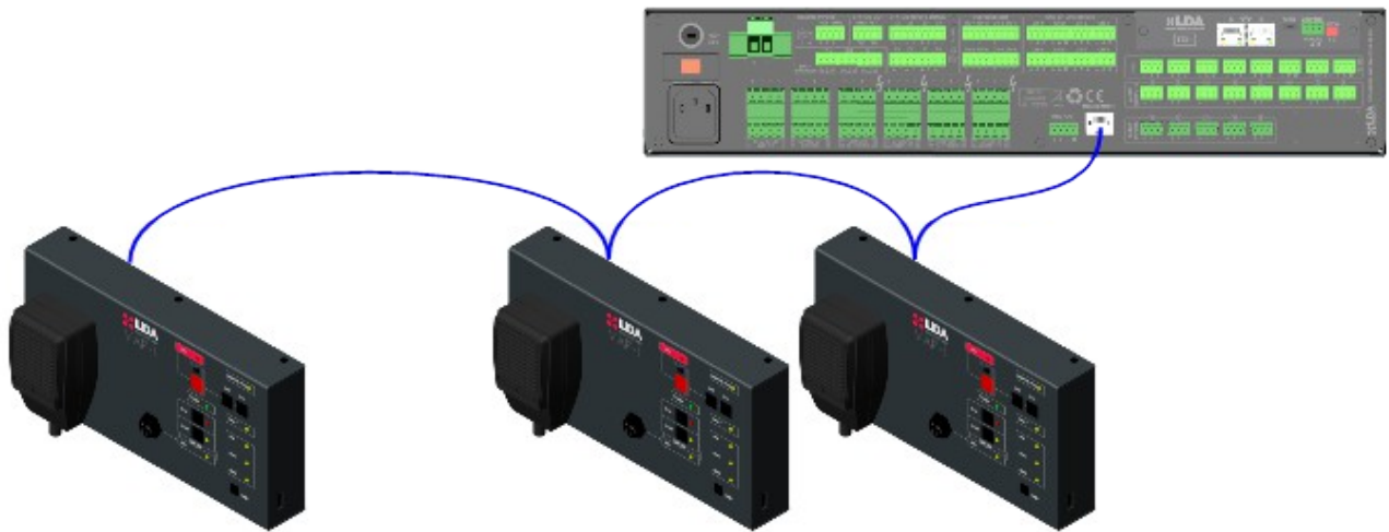
Illustration 9: Connection to the system of voice evacuation
