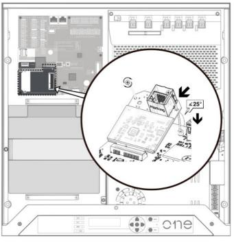
3.- Insert the ONELOOP Module at 25° into the connector, rotate until it is parallel to the motherboard, insert the M2x6mm screws using the Phillips screwdriver "PH1" provided in the box.
