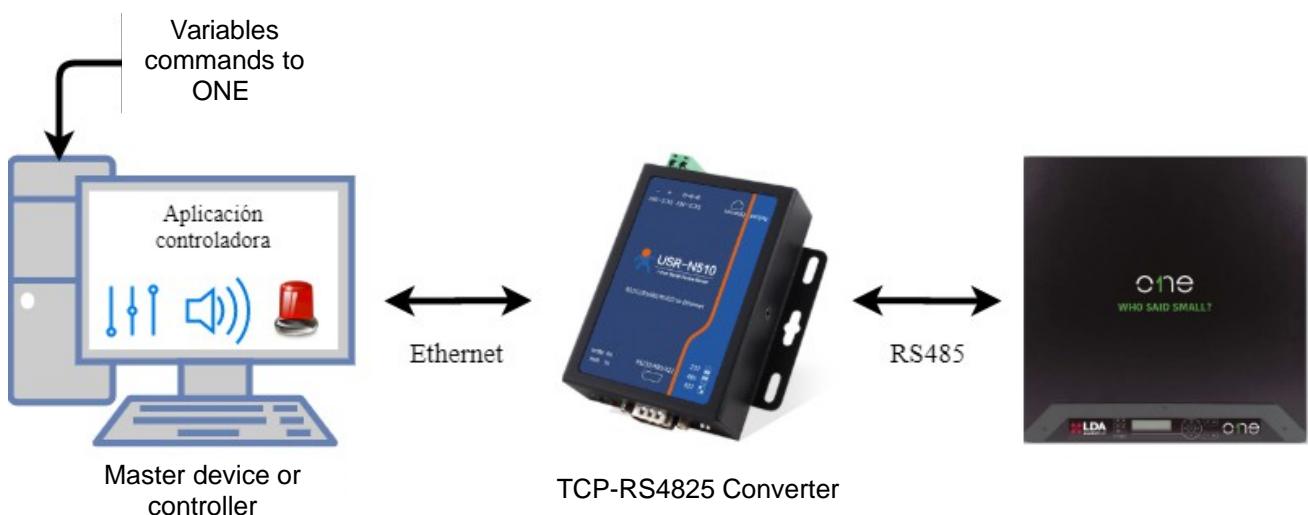
Picture 2: Communication performance between MODBUS RTU and ONE
