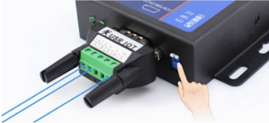
Picture 4: Switch disposition to RS-485 performance
