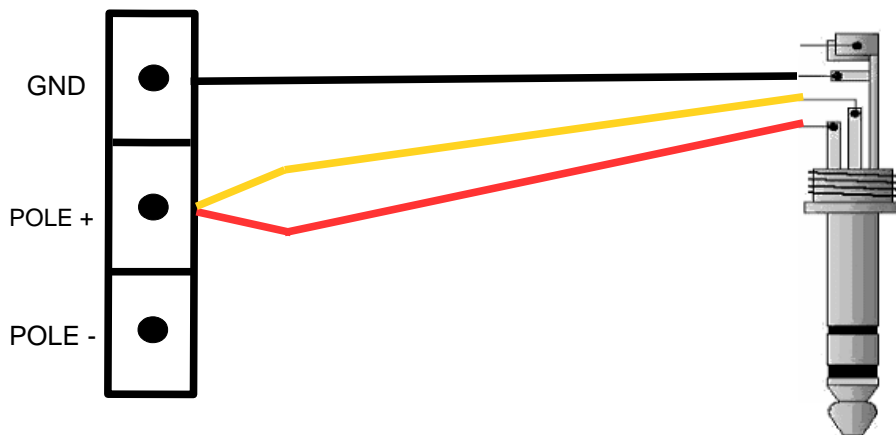
Diagram 3: Balanced audio output connection to Jack
